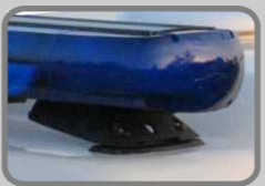
Permanent roof mount
