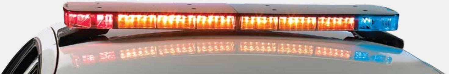
While operating in three priority modes, all modules keep sequence with the flash pattern. Once directional warning is selected, the SignalMaster modules override the current flash pattern.
